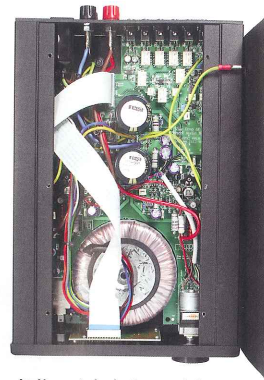
An Alps motorised volume control can be seen bottom right, and to its left a big toroidal mains transformer. Input relay switching is used.
